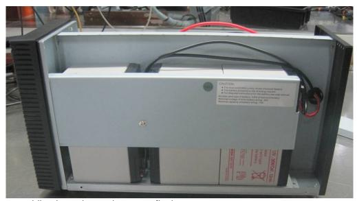
So you finish assembling batteries and you can fix the cover now.
